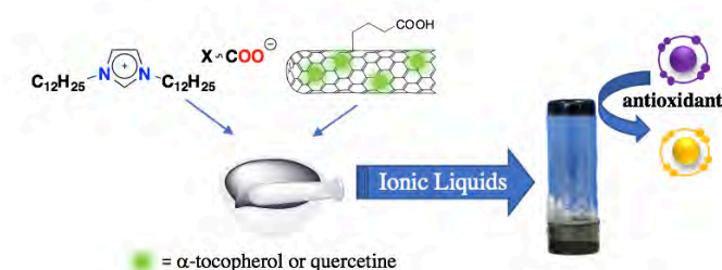
Figure 1. Schematic representation of gelators and CNTs used to form hybrid gels.
